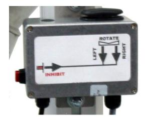
Control Module -Rotate Right/Left Push Buttons -"Inhibit" Button Activation Required Before Rotation of Pail
