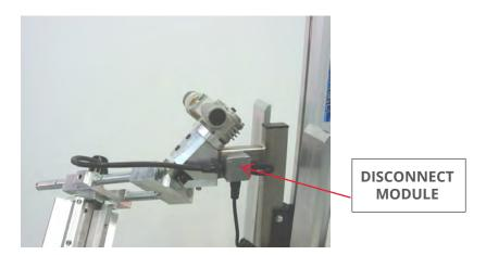
The Quick Disconnect Module provides power to the expander and rotate motor and can be provided with quick exchange features for change out of the expander (different sizes) without changing the complete end-effector for another. When in need of changing expanders, simply unscrew the connection to the module, remove the expander, install the **new** expander and reconnect the power cord to the Quick Disconnect Module.
