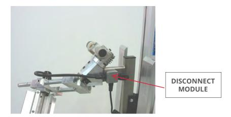
The Quick Disconnect Module provides power to the expander and motor and can be provided with quick exchange features for change out of the expander (different sizes) without changing the complete end-effector for another. When in need of changing expanders, simply unscrew the connection to the module, remove the expander, install the **Bew** expander and reconnect the power cord to the Quick Disconnect Module.
