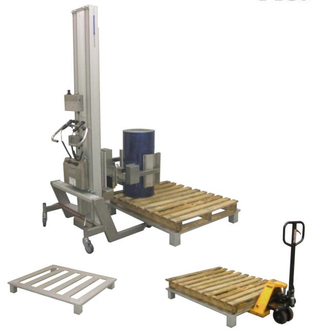
An aluminum posted pallet is used as a workstation to allow LIFT-O-FLEX® ergonomic lifter leg access for loading or unloading wood pallets. Simply place your wood pallet on top of the aluminum pallet. The pallet can now be moved with either a fork truck or pallet jack.
