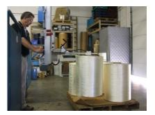
Roll Handling-Expand-O-Turn® Core Vertical to Cores Horizontal
