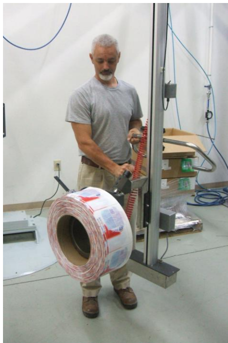
Expand-O-Turn® Air Actuated w/Anti-Telescopic Device-Manual Rotate Roll Handling
