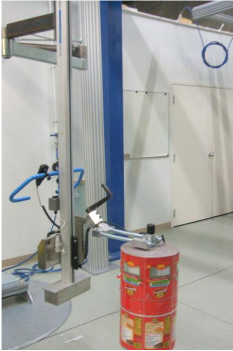
Expand-O-Turn® Electric Expand/Retract Manual Rotate Roll Handling
