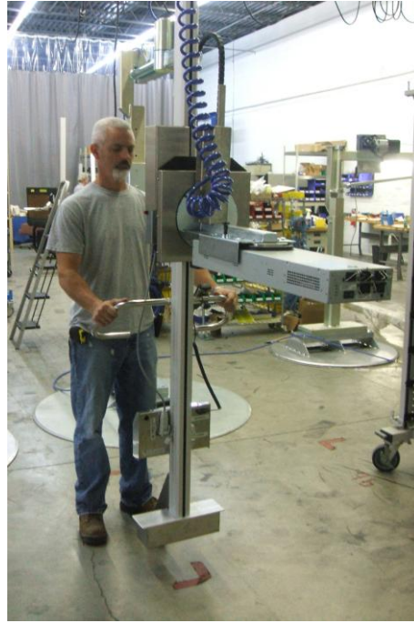
Vacuum Attachment Electric Rotator Plant Air for Vacuum Electronic Handling
